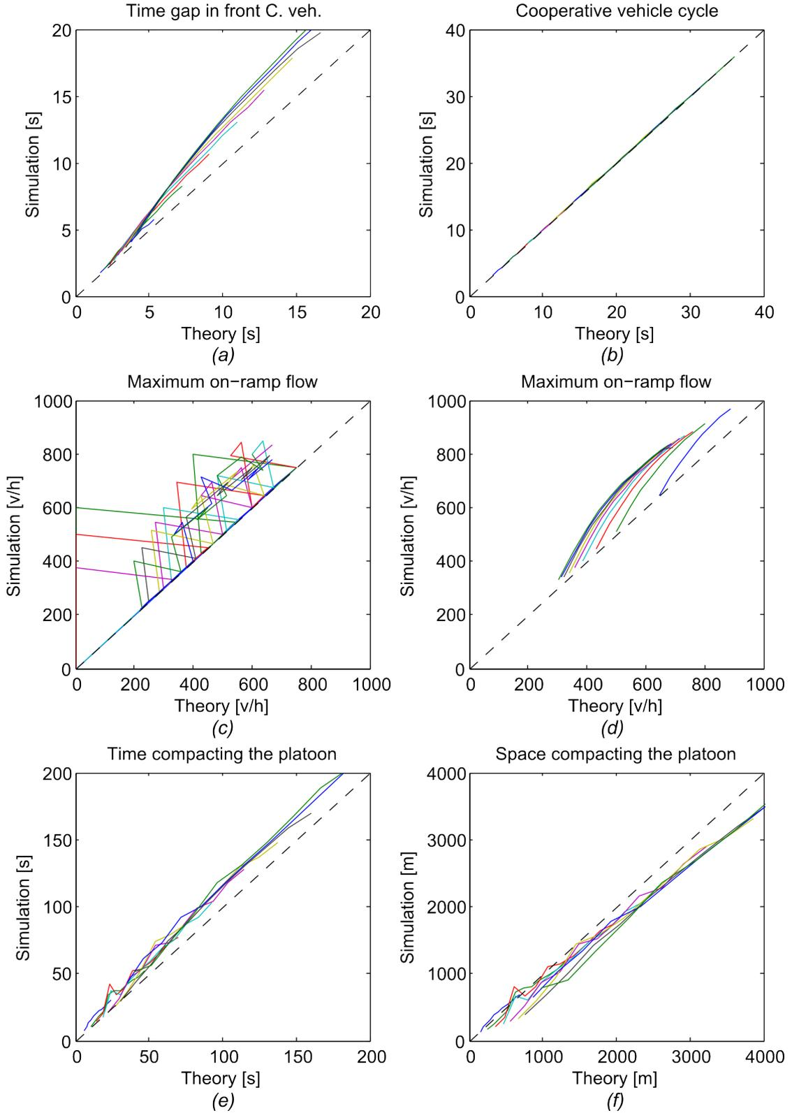
Figure 4.6: Comparison between theoretical and simulation results. (a) gap  $G$  created in front of the cooperative vehicle, (b) cooperative vehicle cycle  $C_c$ , (c) maximum on-ramp flow  $q_0^{\max}$  with the constraint of integer number of vehicles able to merge and (d) without this constraint, (e) time  $t_C$  needed to create the gap and (f) the relative space  $x_C$ .
