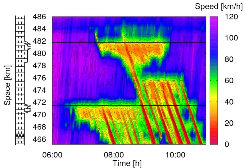
Figure 2.4: Spatio-temporal diagram of the speed with creation of congestion. German motorway A5 southbound - 11 June 2001. Adapted from Treiber and Kesting (2013).
