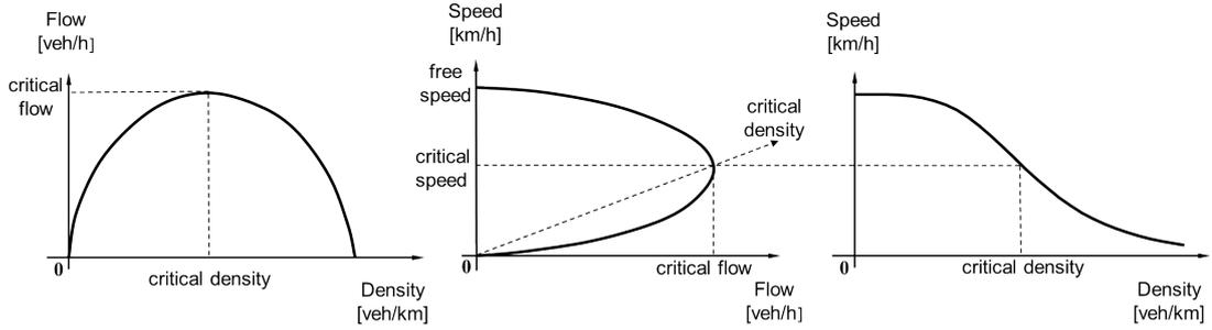
Figure 2.17: Conceptual representation of a classic macroscopic model based on the fundamental diagram of traffic flow.
