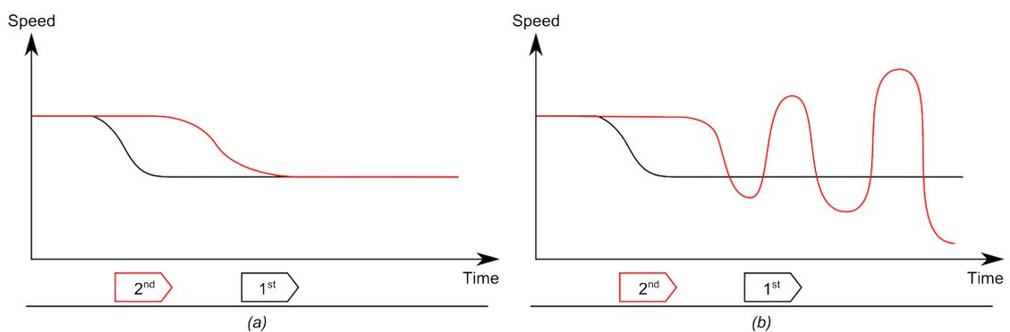
Figure 2.11: Example of local stability in case of (a) stable and (b) unstable situation. Adapted from Pueboobpaphan and van Arem (2010).
