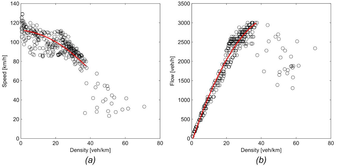
Figure 4.5: VISSIM fundamental diagram and fitted model of the free-flow section.
