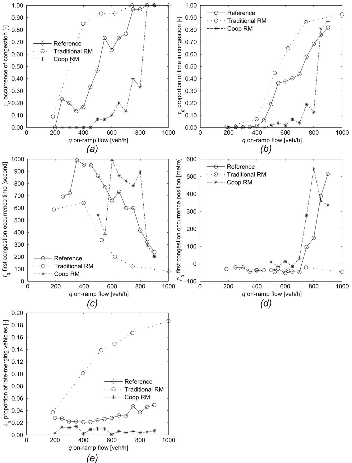
Figure 5.7: Results and comparison for the different simulation threads. (a)  $\gamma_q$  occurrence of congestion, (b)  $\tau_q$  proportion of time spent in congestion, (c)  $t_q$  first congestion occurrence time, (d)  $p_q$  first congestion occurrence position and (e)  $\lambda_q$  proportion of late-merging vehicles.
