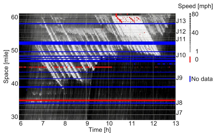
Figure 2.5: Real data spatio-temporal diagram of the speed with presence of missing and inconsistency data. MIDAS data - English motorway M25 Clockwise - 1 May 2002.
