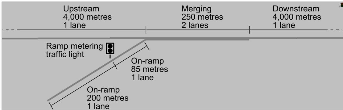
Figure 5.3: Simulated infrastructure of the motorway junction using VISSIM (configured right-hand traffic). The junction is composed of: upstream, merging, downstream and on-ramp links with traffic light.
