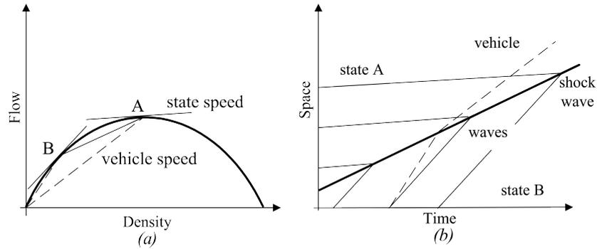
Figure 2.6: Graphical representation of the shock wave theory. (a) shows the fundamental diagram with vehicle speed, state speed and front speed. (b) presents the spatio-temporal diagram with the front propagation. Adapted from Lighthill and Whitham (1955).
