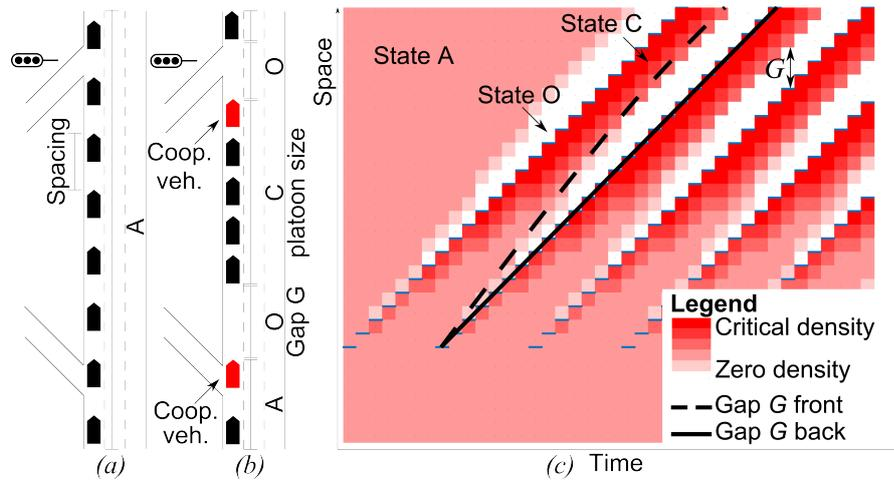
Figure 3.1: Conceptual representation of the effects on traffic flow under Cooperative Ramp Metering. (a) vehicle configuration if CoopRM is not applied, and (b) if CoopRM is applied with creation of platoons and gaps. (c) representation of the spatio-temporal evolution of the main carriageway vehicle density with formation and evolution of gaps  $G$  suitable for merging due to the decrease in speed of the cooperative vehicles.
