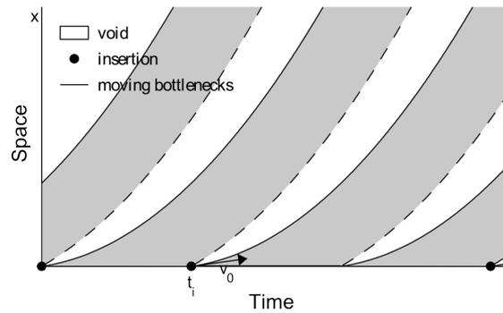
Figure 2.9: Graphical representation of the moving bottleneck concept. Merging vehicles with slow speed create voids in the main carriageway traffic. Adapted from Leclercq *et al.* (2011).
