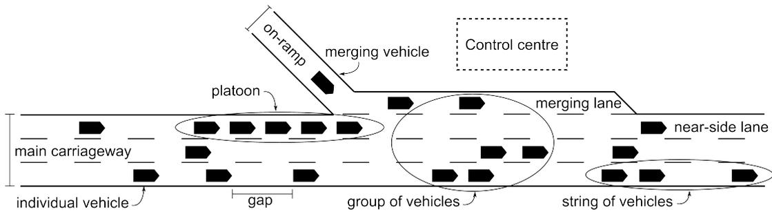
Figure 2.22: Graphical representation of the components involved in the merging process of controlled intelligent vehicles.
