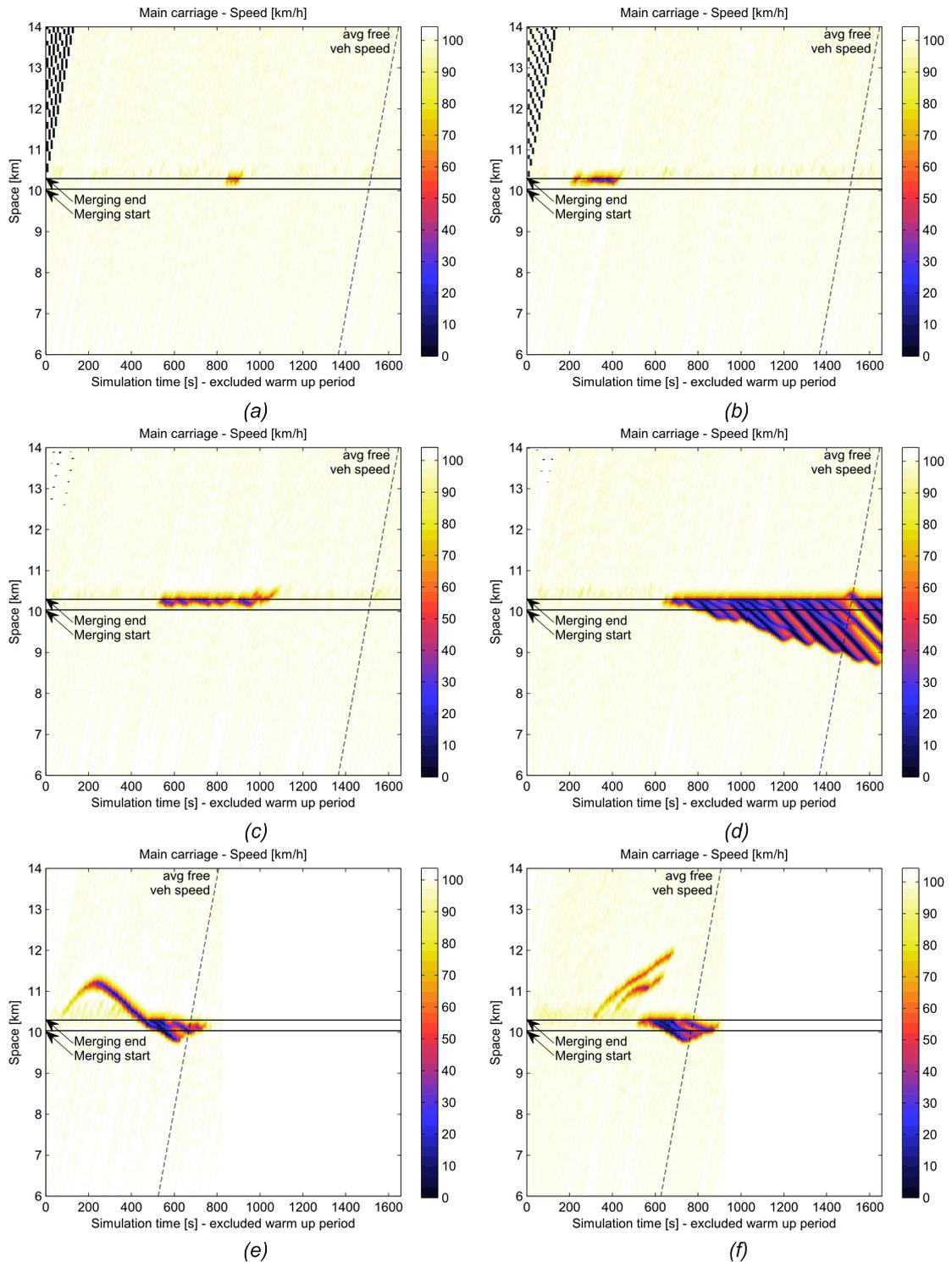
Figure 5.5: Spatio-temporal diagrams of different congestion formation for the Reference scenario. (a) perturbation not classified as congestion (on-ramp flow 200 veh/h, run 1). (b) small congestion (on-ramp flow 250 veh/h, run 11). (c) more severe congestion (on-ramp flow 450 veh/h, run 7). (d) break-down and shock wave formation (on-ramp flow 450 veh/h, run 15). (e) boomerang effect (on-ramp flow 800 veh/h, run 1). (f) perturbation not leading to break-down (on-ramp flow 800 veh/h, run 5).
