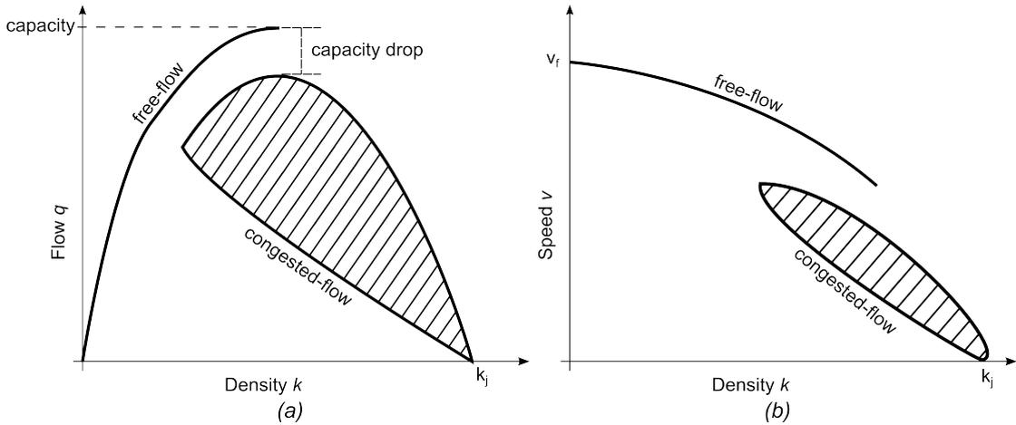
Figure 2.2: Conceptual representation of the fundamental diagram of traffic flow. (a) flow-density plane, and (b) speed-density plane.
