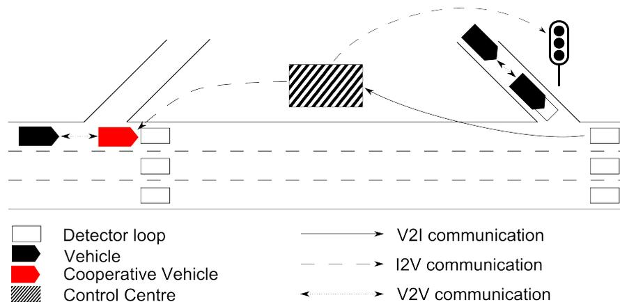
Figure 3.2: Representation of the communication request by the Cooperative RM system. The control centre estimates the traffic conditions on the on-ramp and main carriageway, releases the on-ramp vehicles using the traffic signal and slows down the cooperative vehicle on the main carriageway.
