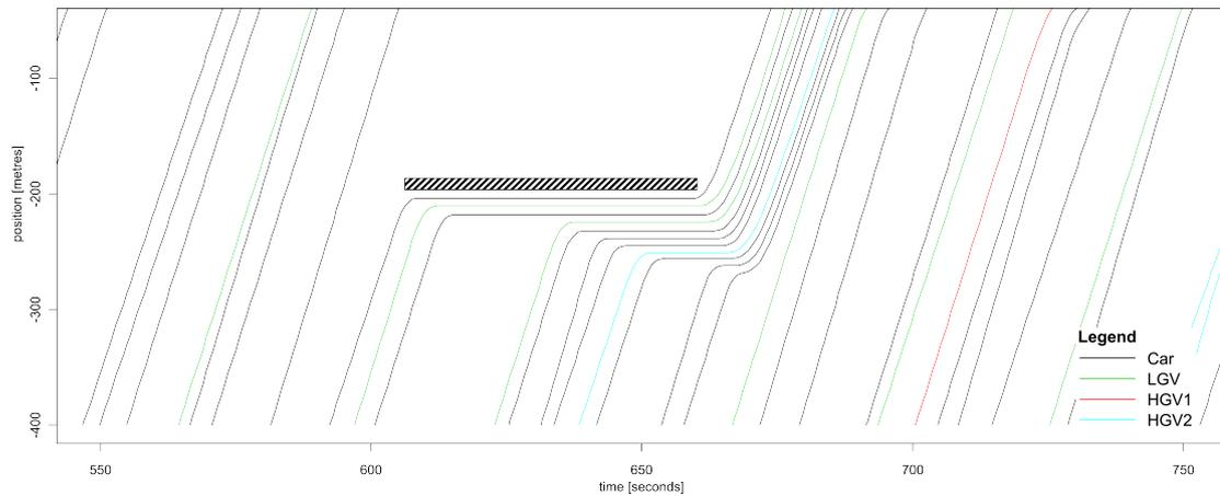
Figure 2.14: Multi modal vehicles trajectory on a single lane, with obstacle, produced by Gipps' car-following model. Simulation data.
