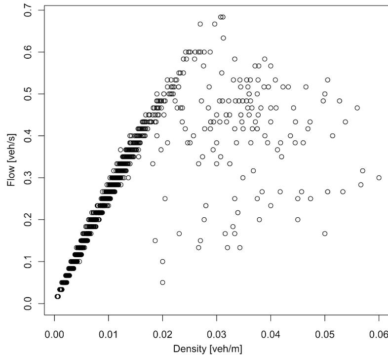
Figure 2.7: Real data fundamental diagram showing an active bottleneck with representation of capacity drop. MIDAS data - English motorway M6 J18 - south-bound near-side lane.
