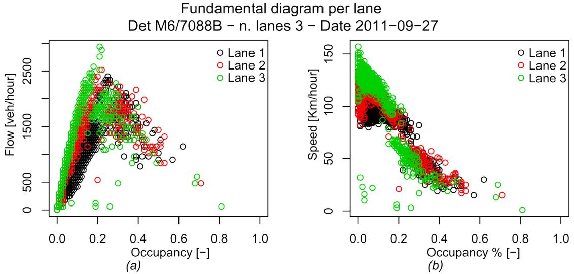
Figure 2.3: Real data fundamental diagram from detector loops in proximity of an active bottleneck. (a) flow-occupancy plane, and (b) speed-occupancy plane. MIDAS data.
