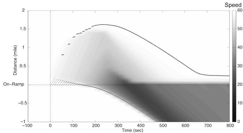
Figure 2.13: Graphical representation of the boomerang effect. Disruptions created at on-ramps eventually lead to break-down downstream of the merging location. Adapted from Kim and Coifman (2013).
