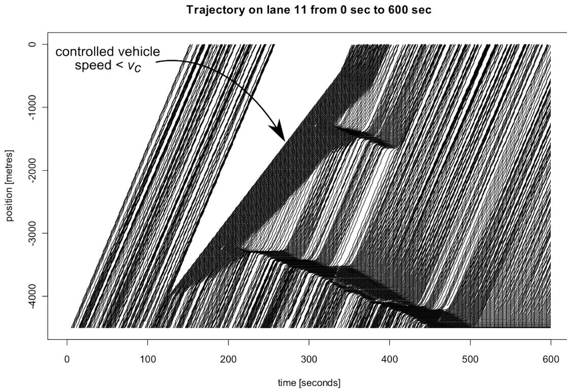
Figure 2.10: Example of supercritical perturbation. Vehicle trajectories in case a vehicle slows down and formation of queue. Simulation data.
