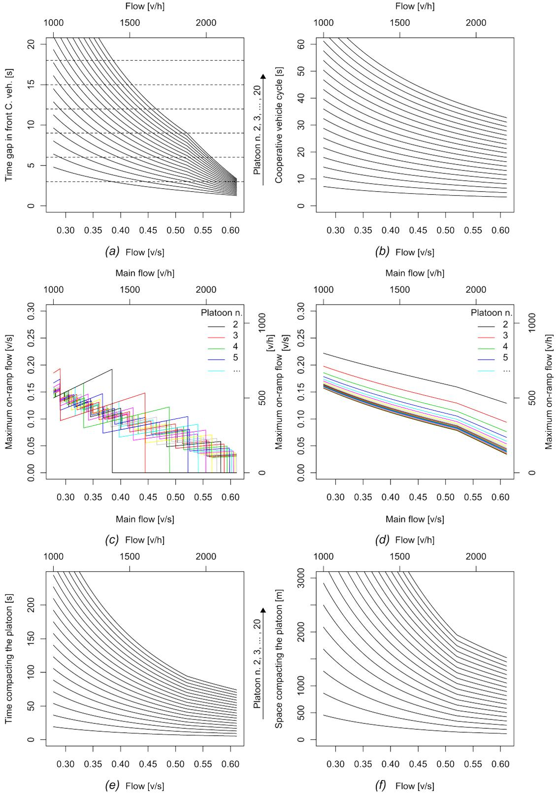
Figure 3.6: CoopRM formulation main results. (a) gap  $G$  created in front of the cooperative vehicle, (b) cooperative vehicle cycle  $C_c$ , (c) maximum on-ramp flow  $q_o^{\max}$  with the constraint of integer number of vehicles able to merge and (d) without this constraint, (e) time  $t_C$  needed to create the gap and (f) the relative space  $x_C$ .
