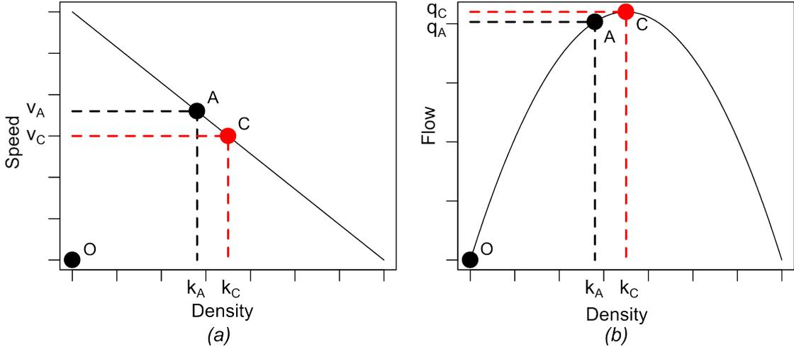
Figure 3.3: CoopRM traffic states. (a) speed-density and (b) flow-density diagrams with the representation of the different traffic state created by the cooperative vehicle.
