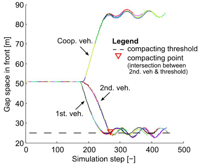
Figure 4.3: Evolution of the clearance in front of vehicles during platoon formation for each simulation step and procedure used to calculate the indexes.
