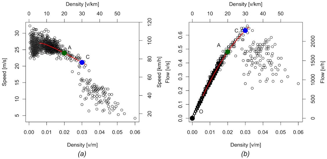
Figure 3.4: Detector loop data (MIDAS English motorway M6-J19) and fitted model with the representation of the actual  $A$  and cooperative  $C$  traffic states. (a) speed-density and (b) flow-density plane.
