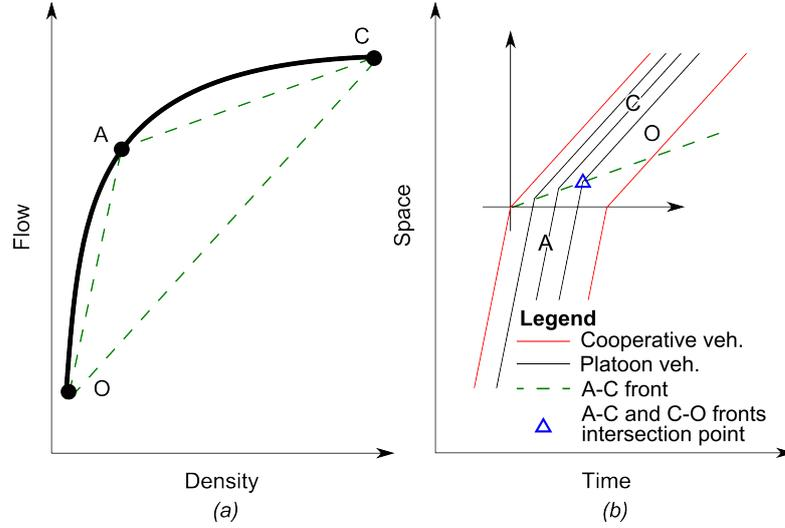
Figure 3.5: Trajectories of the CoopRM traffic state fronts. (a) conceptual illustration of the flow-density fundamental diagram and representation of the front propagation speed. (b) conceptual spatio-temporal diagram of the vehicles trajectory during the different traffic states with representation of the fronts between the states  $A$ ,  $C$  and  $O$ .
