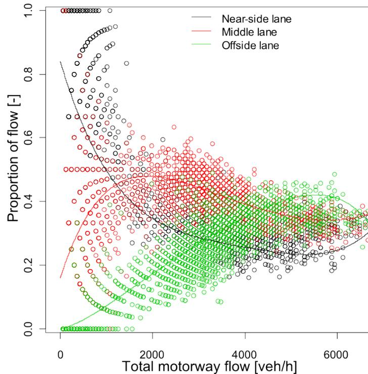
Figure 2.12: Lane utilization factor for an English motorway and fitted model. MIDAS data - English motorway M56 - J2. Model adapted from Al-Obaedi (2011).
