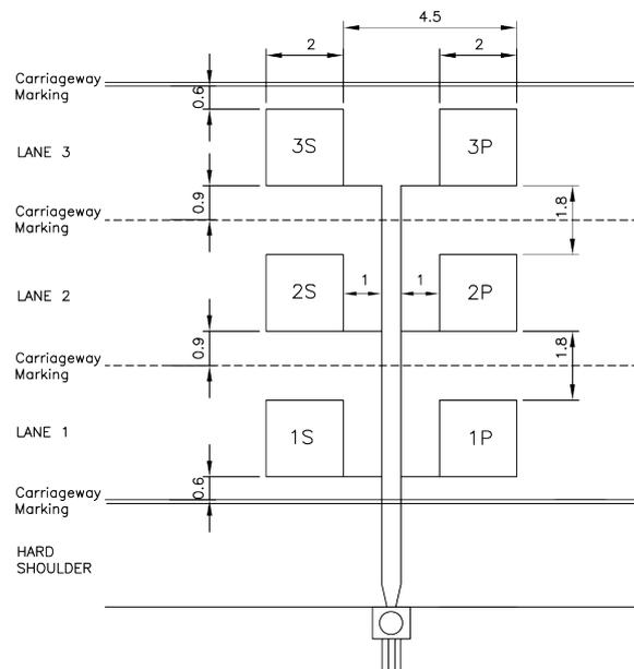
Figure 2.23: MIDAS system detector loop configuration - dimension in metres. Adapted from DfT (2011a, Volume 3, Section 1, Series G).
