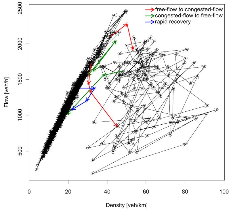
Figure 2.8: MIDAS fundamental diagram with transitions from free-flow to congested-flow and hysteresis phenomenon. MIDAS data - English motorway M6-J18 - southbound near-side lane.
