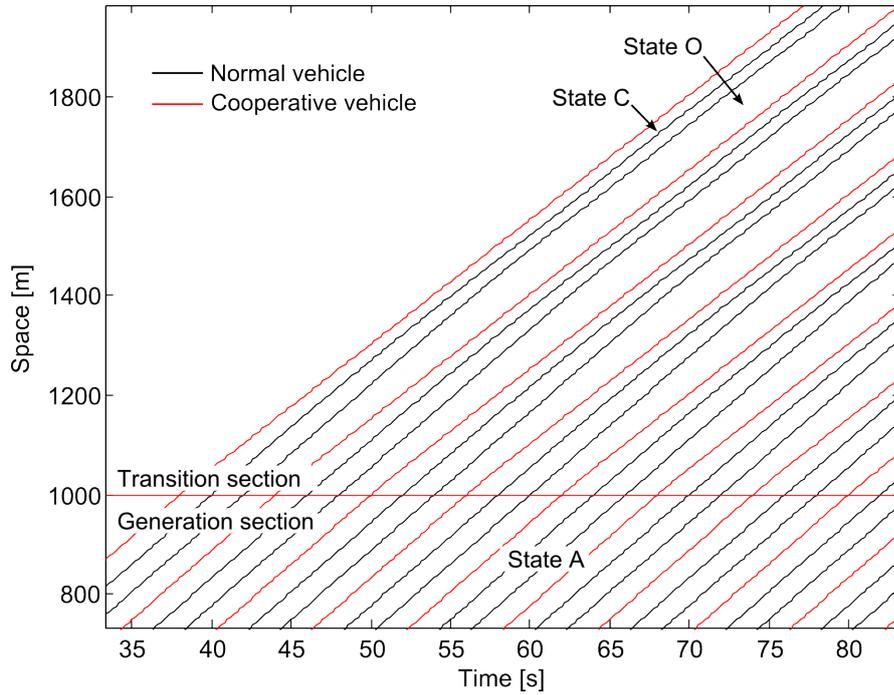
Figure 4.2: Vehicle trajectories in case of a three vehicle platoon with change from state  $A$ , to states  $C$  and  $O$ .
