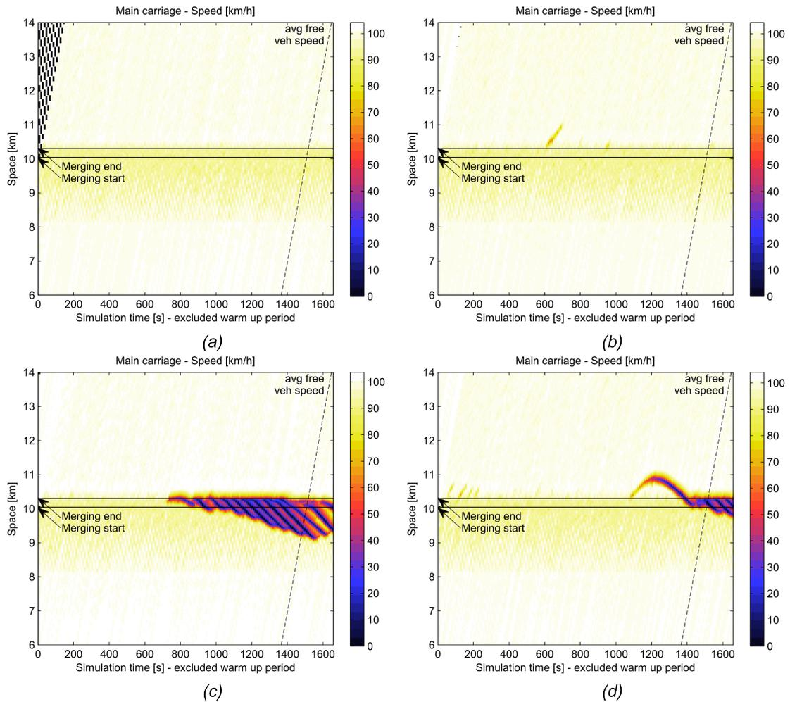
Figure 5.6: Spatio-temporal diagrams of different congestion formation for the Cooperative Ramp Metering scenario. (a) complete absence of congestion and visible cooperative area (on-ramp flow 200 veh/h, run 1). (b) small perturbation not classified as congestion (on-ramp flow 650 veh/h, run 18). (c) break-down and shock wave formation (on-ramp flow 650 veh/h, run 11). (d) boomerang effect (on-ramp flow 750 veh/h, run 23).
