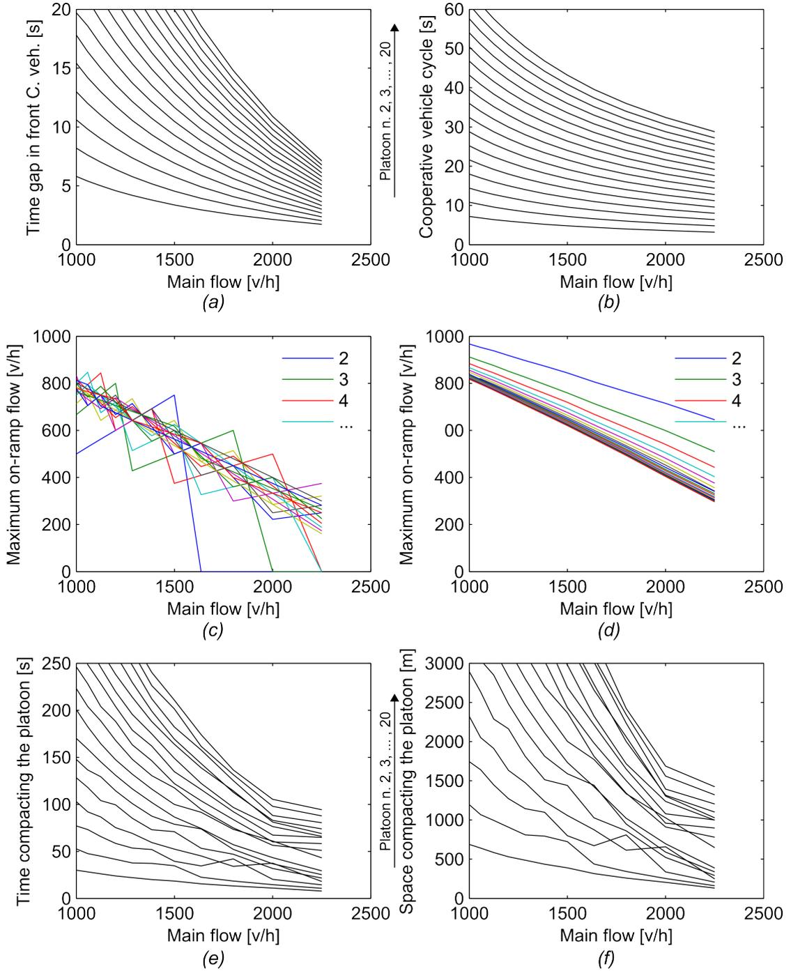
Figure 4.4: CoopRM formulation results obtained by simulation. (a) gap  $G$  created in front of the cooperative vehicle, (b) cooperative vehicle cycle  $C_c$ , (c) maximum on-ramp flow  $q_o^{\max}$  with the constraint of integer number of vehicles able to merge and (d) without this constraint, (e) time  $t_C$  needed to create the gap and (f) the relative space  $x_C$ .
