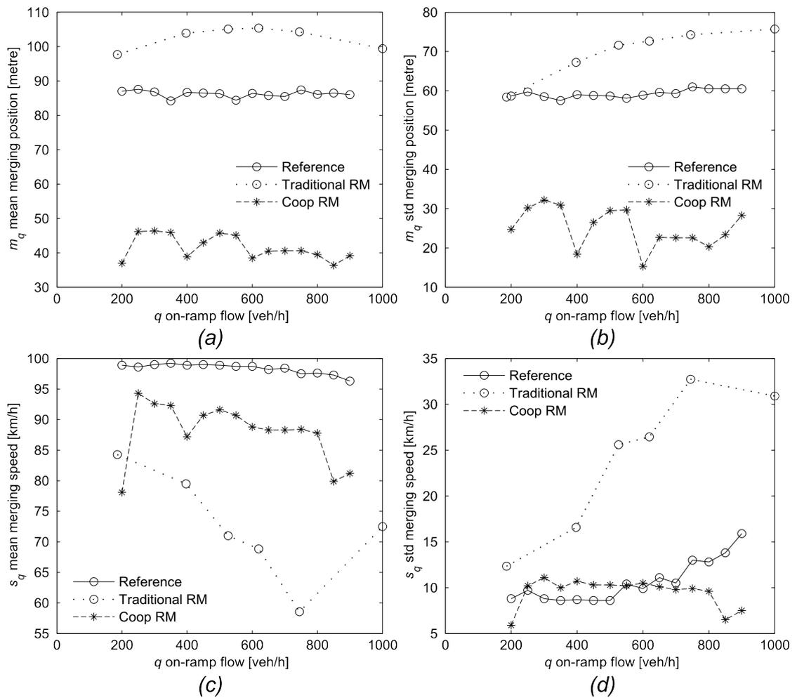
Figure 5.8: Results and comparison for the different simulation threads. (a) mean and (b) standard of the merging position  $m_q$ , (c) mean and (d) standard deviation of the merging speed  $s_q$ .
