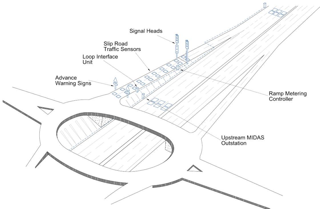
Figure 2.21: Schematic representation of a standard English motorway junction equipped with a RM system. Adapted from HA (2007b).
